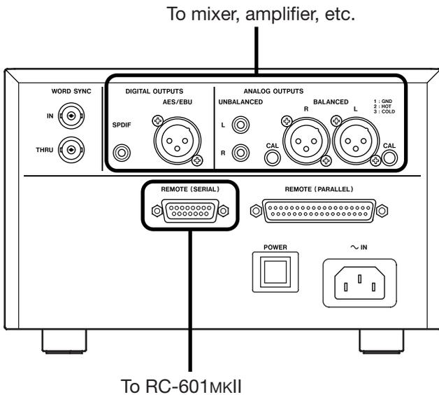
If you have the RC-601MKII remote control unit, connect the **PLAYER UNIT** port on the RC-601MKII rear panel to the **REMOTE (SERIAL)** port on the CD-601MKII rear panel using the cable supplied with the RC-601MKII.
