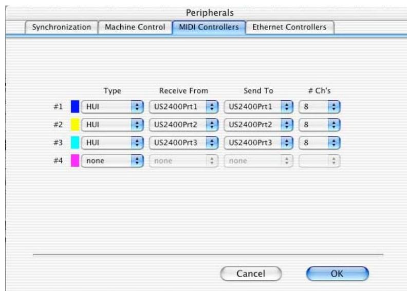
5. Set the Type of controllers #1-3 to HUI. Set the rest of the controls to match the ones above. For example, HUI #1 receive from US2400Prt1 and send to US2400Prt1.
