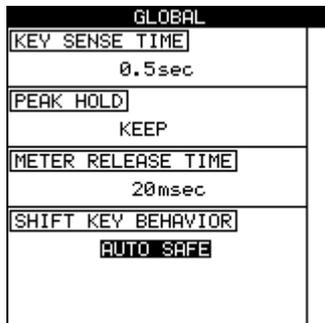
**Key sense time** Some of the keys on the unit have two different functions, depending on whether they are pressed and released in a short space of time, or whether they are pressed and held down for a longer period.
