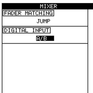
**Fader matching** The option affects the way in which the physical and the virtual faders interact (see “Faders” on page 24). There are three options here:
