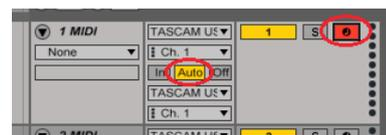
If you play a MIDI keyboard or a MIDI pad connected to the MIDI IN terminal of the US-2x2 in this condition, the meter on the left of the input MIDI channel lights in yellow. This is the input meter, which indicates that a MIDI signal is input into this track. The meter on the right side is the output meter of the track and lighting in yellow of the meter indicates that a MIDI command is output from the track.
