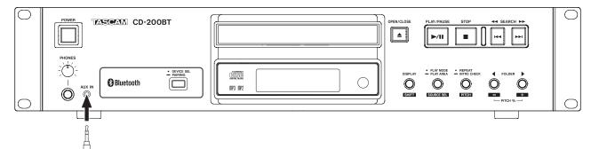
By connecting the audio output of a portable music player or similar device to the external input (**AUX IN**) jack, the audio from that device can be output from this unit's output jacks. The level input through the **AUX IN** jack cannot be adjusted by this unit. Adjust the output level of the external device.
