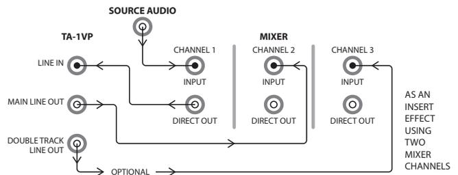
For this configuration, your mixer must provide direct channel outputs.
