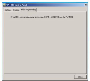
To enter MIDI Programming mode, hold SHIFT and press the MIDI CTRL key; the MIDI CTRL key will blink. (Note that this will only work if the FW-1884 is connected to a host computer.) The FW-1884's Control Panel will open to the MIDI PROGRAMMING tab. (You can leave MIDI Programming mode at any time by pressing the MIDI CTRL key again or selecting any other control surface mode.)
