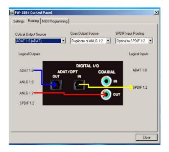
**Optical Output Source** This menu selects the source of the audio output appearing at the FW-1884's ADAT optical outputs. The selections are:
