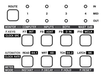
While in MIDI routing mode, selecting any input key will display its selected MIDI outputs. Additionally, all MIDI indicator LEDs will glow steadily to display routing information.
