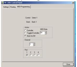
To change the MIDI output(s): Checking or unchecking the four Port boxes will select or de-select the corresponding MIDI output. MIDI messages generated by the key that you're programming will be sent to each port whose associated box is checked. Uncheck all four ports to make a key inactive.
