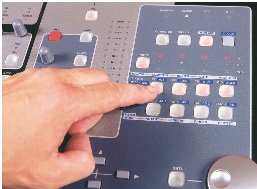
The FW1884 and host sequencer can be switched between different automation modes at the touch of a button.
